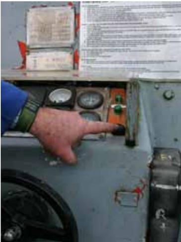
Our launch, “Thumper” has a start button located at the lower right hand side of the instrument panel. Recently, I have observed one or two folk press this button in an attempt to stop the engine as they would in their cars. It’s worth remembering that operation of the starter motor while the engine is running is likely to damage it since “Thumper” has a simple electrical system with none of the safety features to prevent inadvertent operation of the starter motor while the engine is running.
