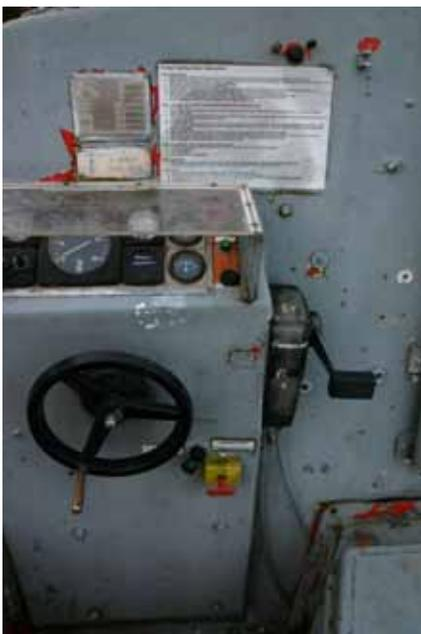
After the engine has stopped, the battery isolator switch (the one into which you fit the key) should be switched OFF, always. Do not leave the battery switched on while the engine is stopped. The horn and bilge pumps circuits remain live when the battery switch is OFF. It’s worth reminding readers that switching the battery off while the engine is running will not shut down the engine but may damage the alternator.
